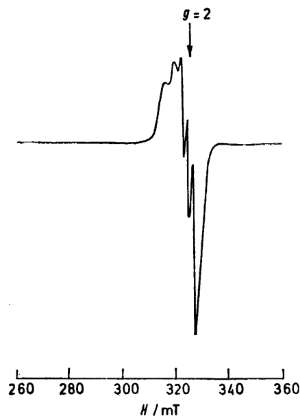
FIGURE 4 E.s.r. spectrum of a frozen aqueous solution (133 K) containing iron(III) tspc ( 5.0 \times 10^{-3} \text{ mol dm}^{-3} ), hydroxylamine hydrochloride ( 5.0 \times 10^{-2} \text{ mol dm}^{-3} ), and 20% v/v dmf at pH 5.0. Microwave frequency 9 149 MHz
